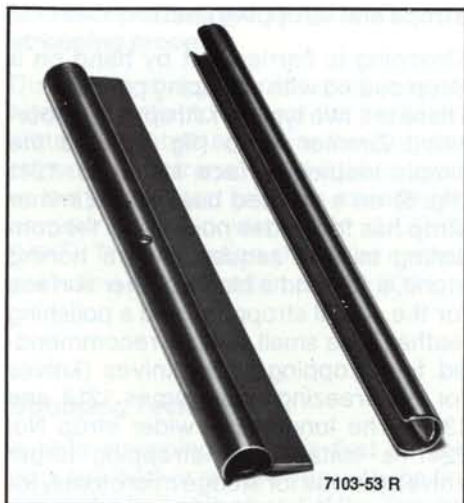
Fig. 2 Stropping bevels, for profile d knives on the left, and for profiles a, b, and c on the right.
