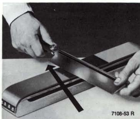
Fig. 6a Illustration of stropping motion (oblique and parallel stropping)
