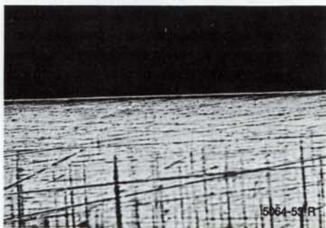
Fig. 7 Microscopic image of a well stropped microtome knife, magnified 200X.
